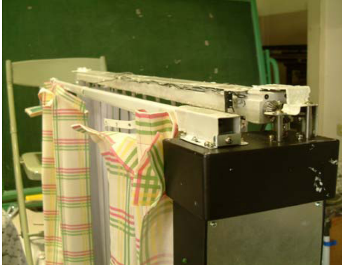
Figure 3: An example of the automatic light-sensitive curtain.
