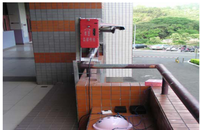
Figure 2: A fully automatic canopy controlling module.
